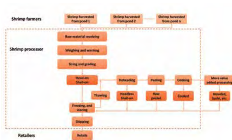
Fig. 10 Flow chart of shrimp processing, system boundary for LCA analysis
