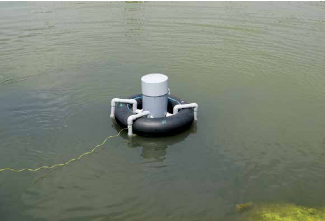
Aqua Buoys embedded with sensors
